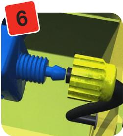
The AQUAvalve can now be connected to the 6mm pipe. Unscrew the yellow collar and push the pipe through it. Push the 6mm pipe onto the nozzle of the AQUAvalve and then replace the yellow collar by screwing it onto the AQUAvalve.
