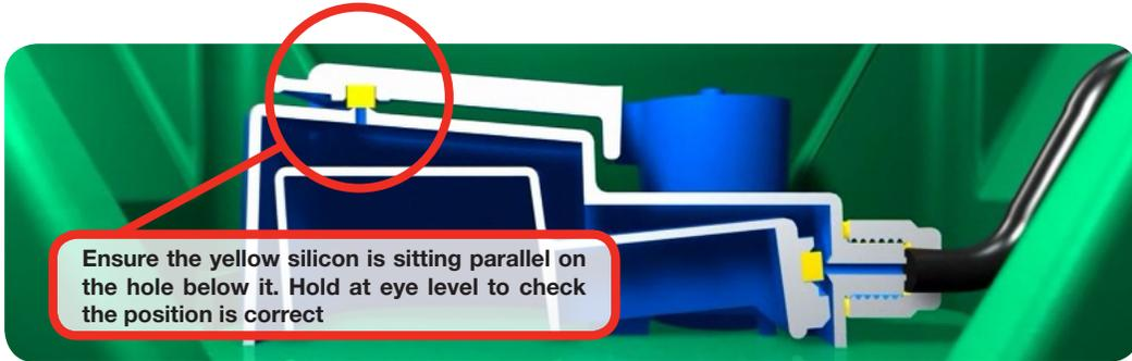
Ensure the yellow silicon is sitting parallel on the hole below it. Hold at eye level to check the position is correct
